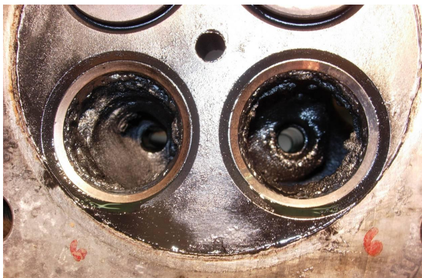
Picture 5: Air inlet port operated 2.900 h on rapeseed oil 31
