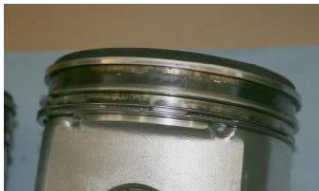
Picture 9: Piston without sediments and free piston rings 36
