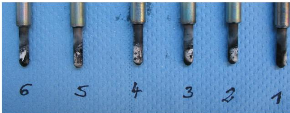
Picture 12: Glow plugs with phosphorus sediments 39
