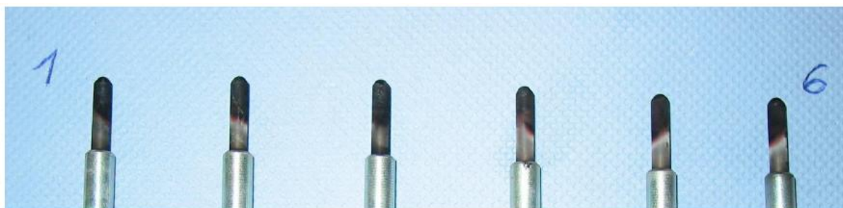
Picture 13: Glow plugs without phosphorus sediments 40
