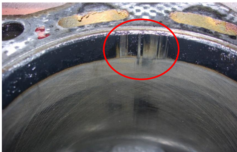
Picture 2: Cylinder-operation-box, operated 2.900 h with rapeseed oil 27
