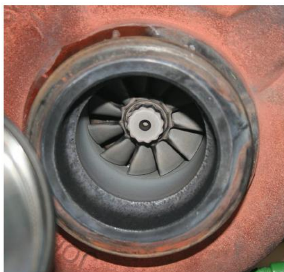
Picture 11: Turbocharger covered with typical black-coloured soot particles 38
