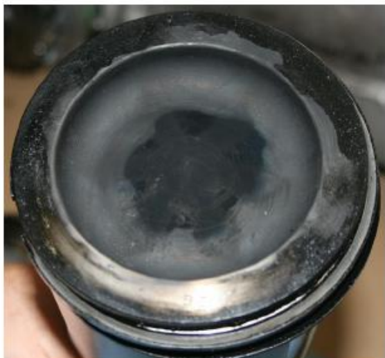
Picture 8: Pistons without sediments 35
