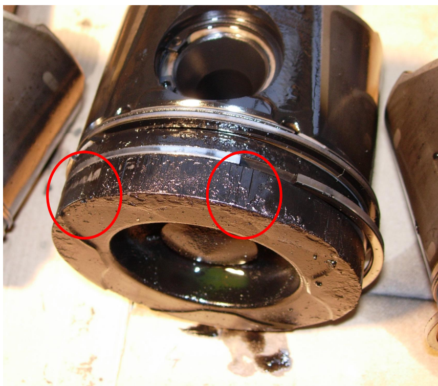
Picture 1: Piston, operated 2.900 h with rapeseed oil 26
