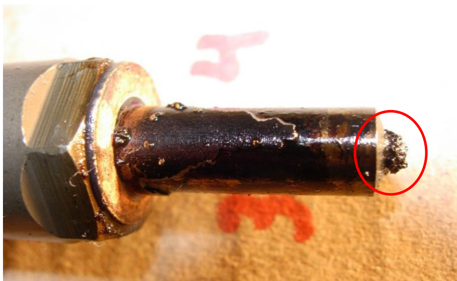
Picture 3: Injection nozzle, operated 2.900 hours with rapeseed oil 28
