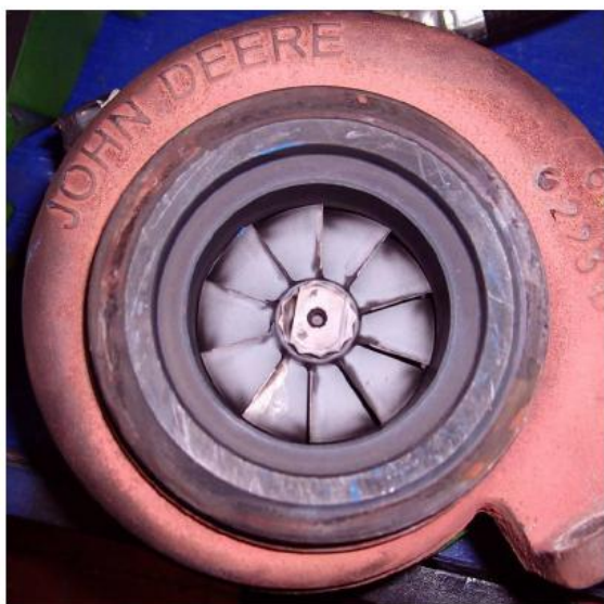
Picture 10: Turbocharger covered with a grey phosphorus layer 37
