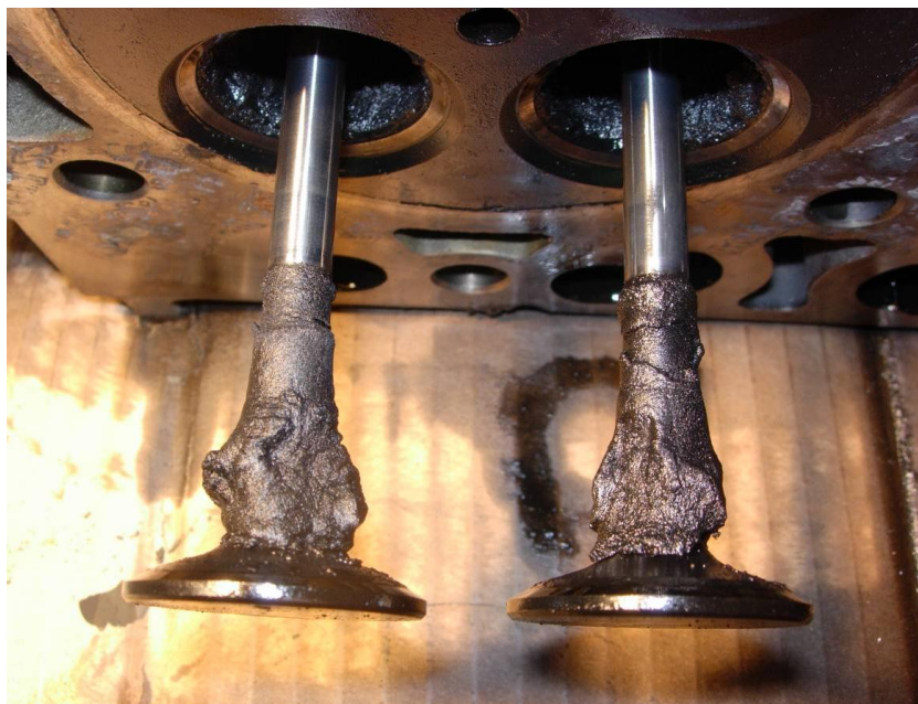
Picture 4: Inlet valves, operated 2.900 h on rapeseed oil 30
