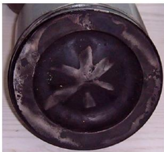
Picture 6: Piston with sediments 33
