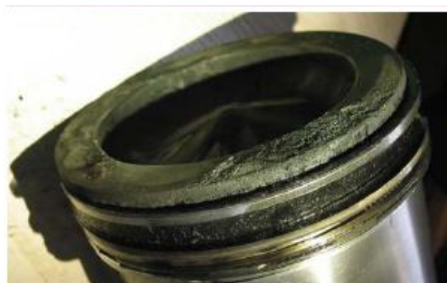
Picture 7: Piston and piston rings with sediments 34
